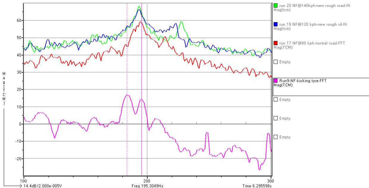
The response (amplitude) inside the tyre is a function of the amplitude of the forcing function. The relatively gentle tap with the foot, to allow the extraction of the cavity mode resonance frequencies is shown to be some 40+dB lower than the running tyre response to road input.
