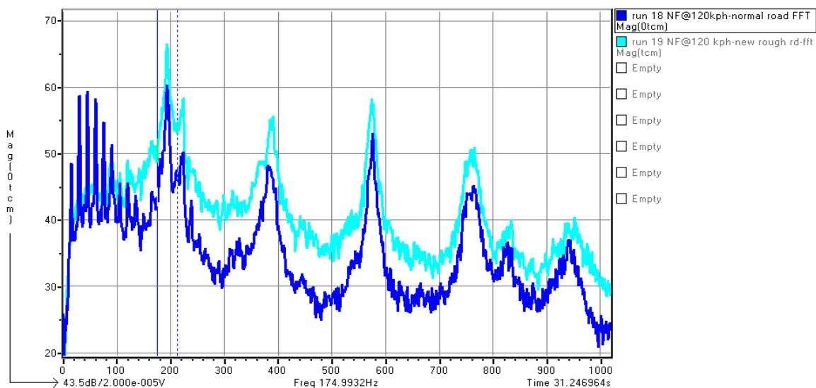
The cabin noise levels reflect the increase in TCM level when going from smooth to rough asphalt for the primary cavity resonance, see figure 11.
