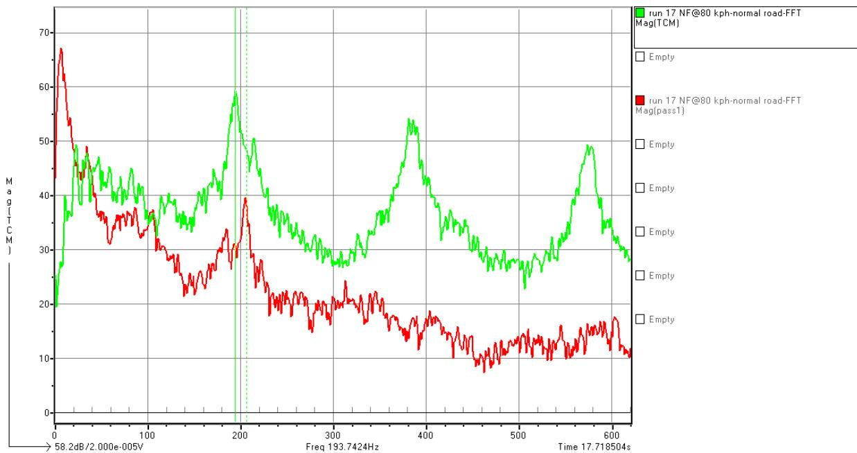
Comparing the in tyre data at the three speeds 140/120/80kph, see figure 5, the frequency of the primary cavity mode can be seen to be constant, within a tolerance of 1Hz.
