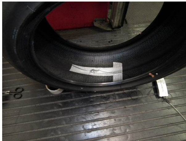
Figure 1. TCA's accelerometer installed on tyre liner
