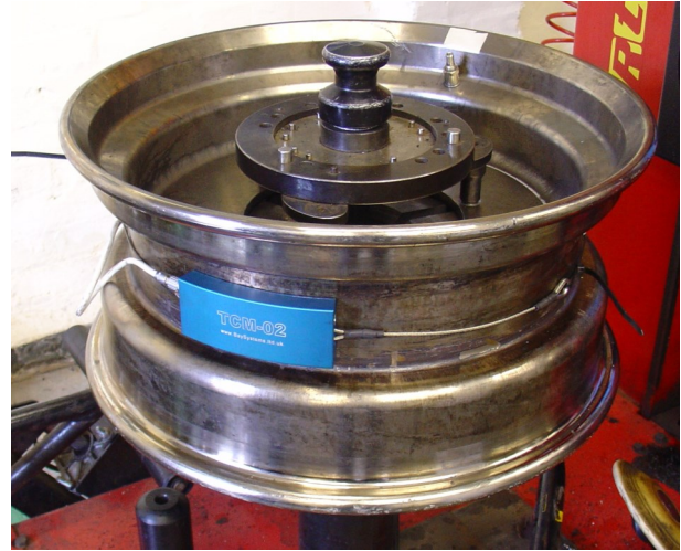
Figure 1. TCM installed on test wheel
