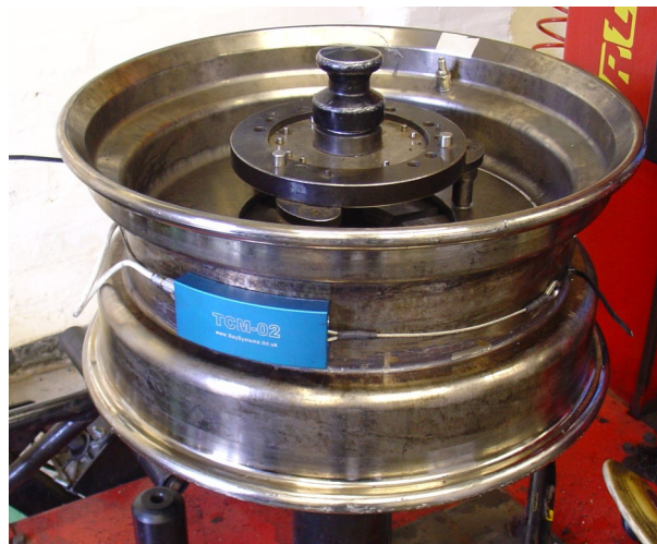
Figure 1. TCM installed on test wheel
