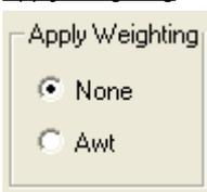
Leq should be calculated with A-Weighting applied. If the signal is already weighted by the acquisition system then “None” should be selected. If A-Weight is required then the signal sample rate must be 44.1KHz or greater. This is to ensure that the digital A-weight filter complied with the IEC651 standard for a Type 1 filter.
