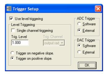
Easy to set up external trigger, e.g. a battery connected to the ADC trigger BNC, or a channel trigger.
