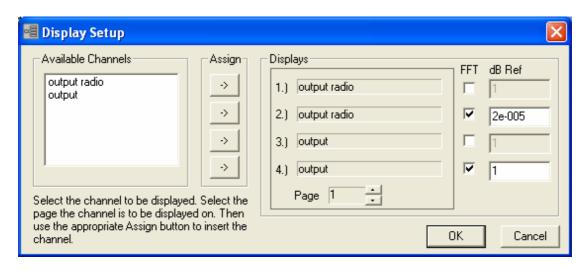
A reference value for each FFT display can now be added. This means that for acoustic measurements the dB can be displayed ref 2E-5 Pascals rather than ref 1Pascal.
