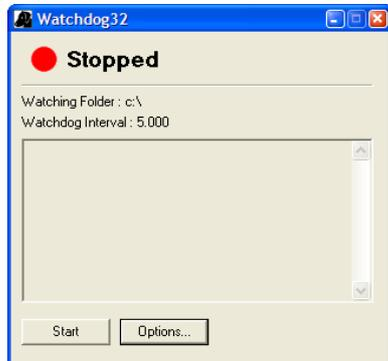
Watchdog is a single panel application that is used to load data from the Sony EX Data Acquisition System. The module monitors a user specified directory for the presence of XMR (Freq domain) and XMX(Time domain) data files. If new files are detected the user has the option to load the file automatically or to be prompted. The Monitoring interval, spectral types and max file load size can be configured by the user.
