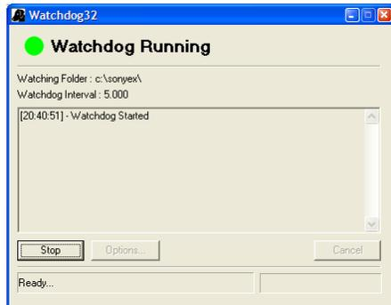
Watchdog is a single panel application that is used to load data from the Sony EX Data Acquisition System. The module monitors a user specified directory for the presence of XMR (Freq domain) and XM(X)Time domain) data files. If new files are detected the user has the option to load the file automatically or to be prompted. The Monitoring interval, spectral types and max file load size can be configured by the user.
