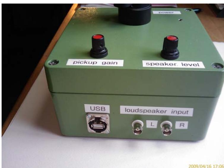
The right hand rotary knob is the output level control for the power amplifier that is driving the loud speaker. If you are resting the pickup on the film over the cup then set this control fully anti-clockwise, the minimum. You should use the computer sound card control to set the output level of the sound card to approximately 3/4 of maximum, this should avoid any distortion inherent with cheap sound cards when driven at maximum level.
