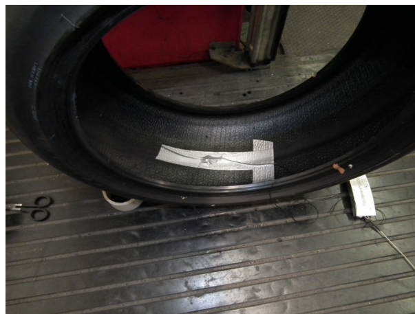
Figure 1. TCA installed on tyre tread liner
