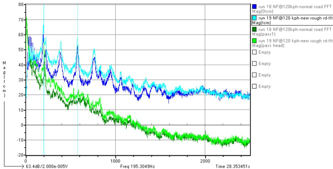
**Tyre primary cavity mode - comparing smooth and rough asphalt surfaces**
