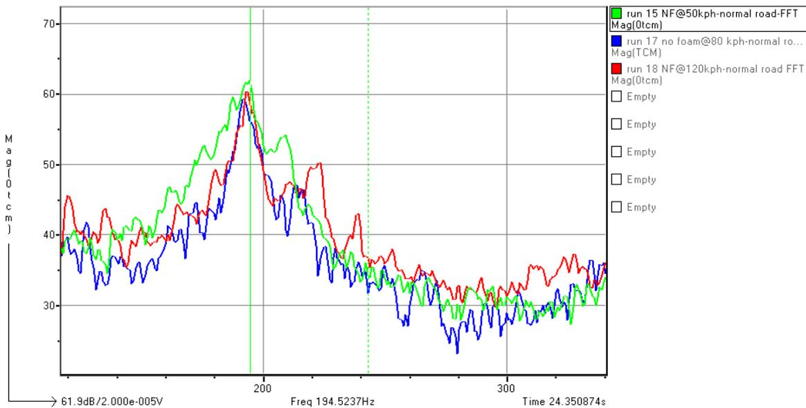
**Figure 8. Cavity resonance frequencies measured inside cabin at 50/80/120kph on smooth asphalt**
