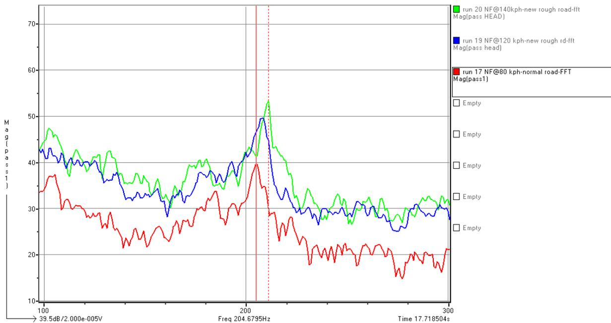
The 80kph run completed on the older smoother asphalt was significantly lower in level than runs completed on the new rough asphalt. Plotting the in tyre and cabin levels for 50/80/120kph for the smooth asphalt reveals that at 50kph the primary cavity resonance is at a greater amplitude than at 80 and 120kph, see figure 7 & 8.
